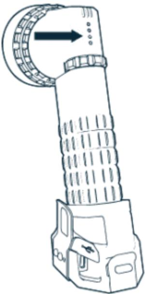
Press the trigger button while Mode Select Dial is in the **Off** position to show battery life.
