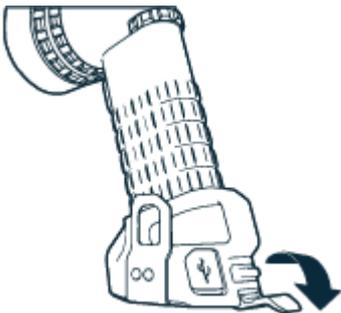
To remove the battery, unlatch the battery cover. After removing the spacer, insert the battery positive (+) side first.
